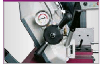
▶ Easy and correct adjustment of the saw band tension
